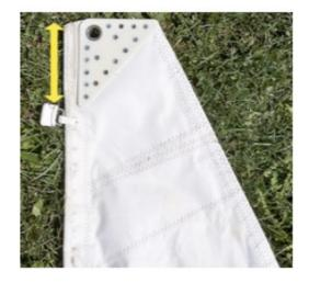
Next, attach two shackles through the two larger holes in the base plate (as shown in photo below right). Use shackles that fit whatever clip or knot you have on the end of your halyard. Connect both shackles to
